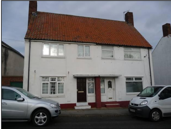
Plate 26. The mismatch of historically inappropriate windows and doors does much to reduce historic character along Bank Top, while the basic architectural proportions and colours of roofing, chimneys and render were designed to fit in. These houses originally matched those on Bishop's Garth but have fared less well with the loss of their traditional windows and doors
